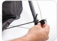
Now set the length of the speed bar. This is best done on a static hang point or alternatively it can be done on the ground. Make sure the speed system is not set too short and that it is symmetrical.
