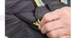
Finally the ends of the nylon pins can be neatened into the available tunnel as shown.
